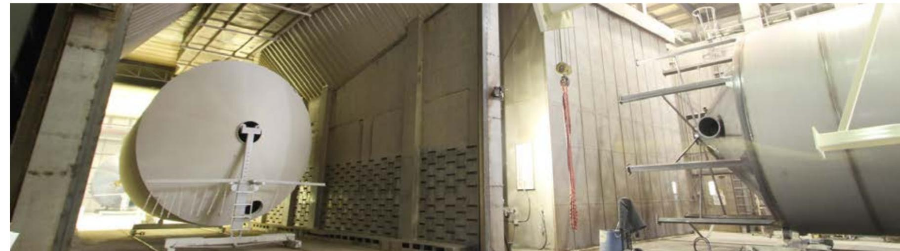
**MERIDIAN'S PRE-ENGINEERED PREMIUM POWDER COAT FINISH** (MPS-1000) has a Salt Spray Rating of more than 2,000 hours, 3-4x more than wet paint standards. The superior adhesion and smooth, long-lasting finish of polyester coating ensures that Meridian SmoothWall Hopper Bins will be incredibly durable and will stand the test of time. Meridian's exterior finish is backed by our 5 Year Paint Warranty.
