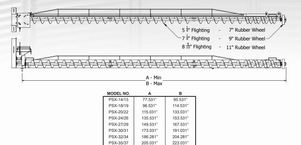
222.531" PSX-42/43 243.531" 261.531" PSX-44/46 260.531" 278.531" PSX-48/50 279.531" 297.531" 'X' identifies size. For correct Model, Substitute 'X' with 5, 7 or 9.
