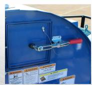
**Inspection Doors** Providing convenient access to inside of head section.
