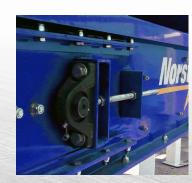
**Slack Adjustment:** All internal lengthening with no increase in actual conveyor length.
