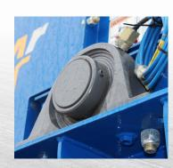
**Head Bearings** Heavy-duty pillow block bearings are externally
